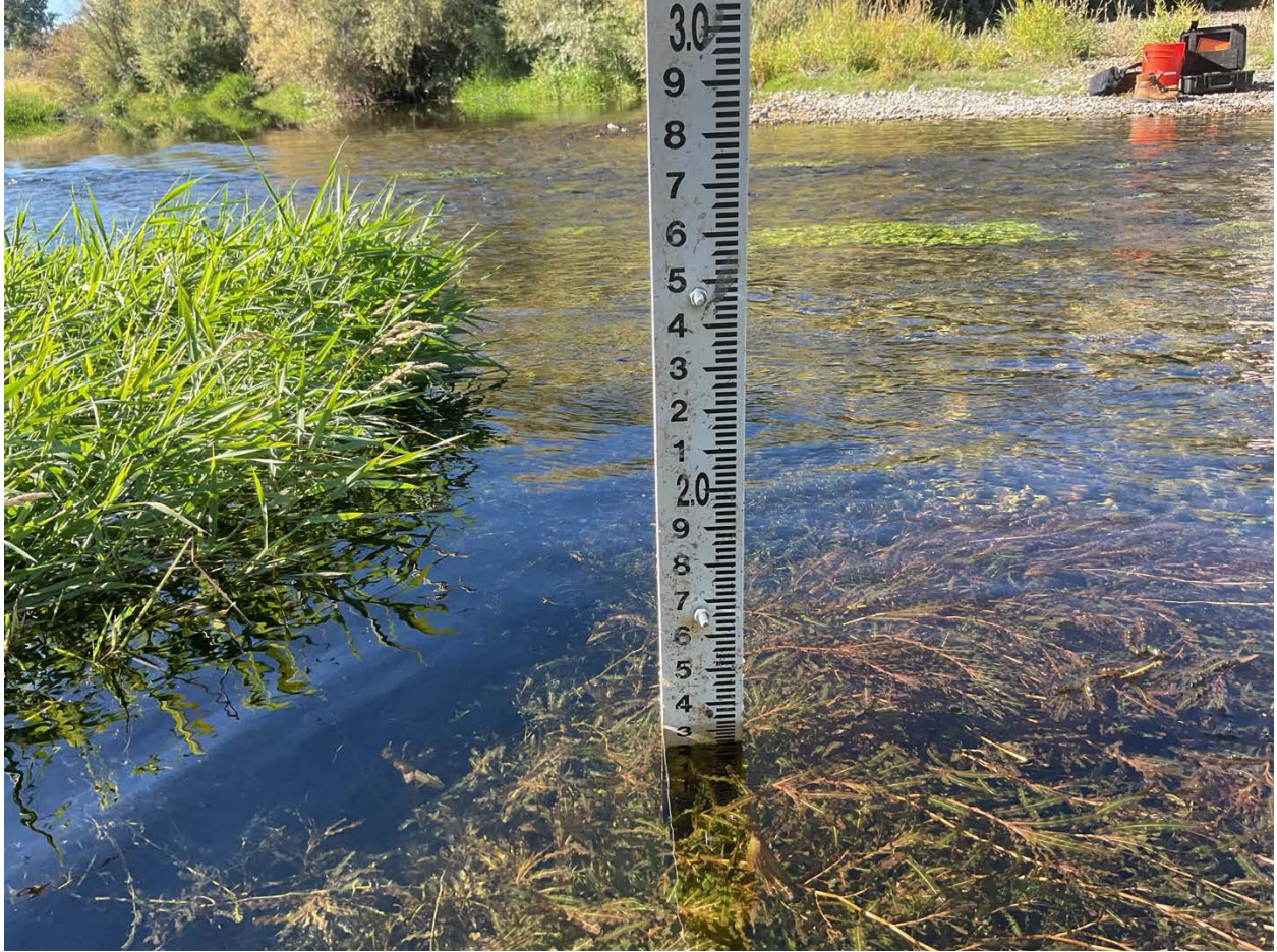
Photo 3: Horn Site Static Staff Gage 1. (SRCD, 2024)
