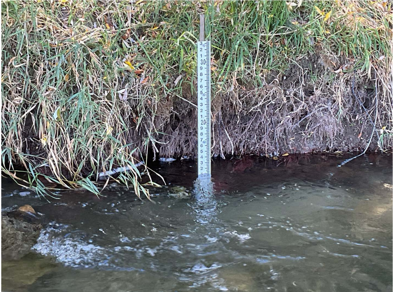
Photo 1: 'Static' In-stream Staff Gage Installation, River-left, Meamber Bridge Site (SRCD, 9/24/24).
