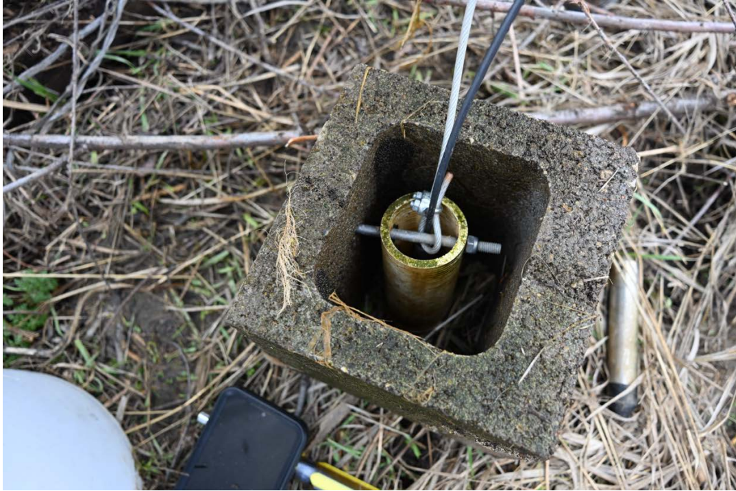
Photo 9: Static staff gage sensor deployment set-up, before wire protection application. (SRCD, 2025).
