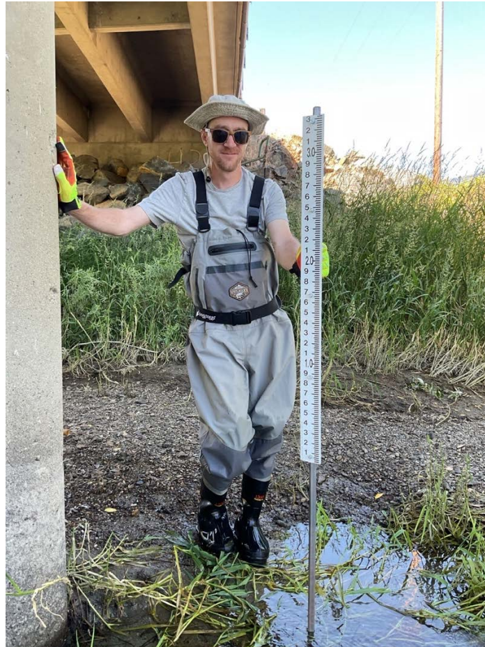
Photo 8: 'Static' staff gage design (SRCD, 6/19/2024).
