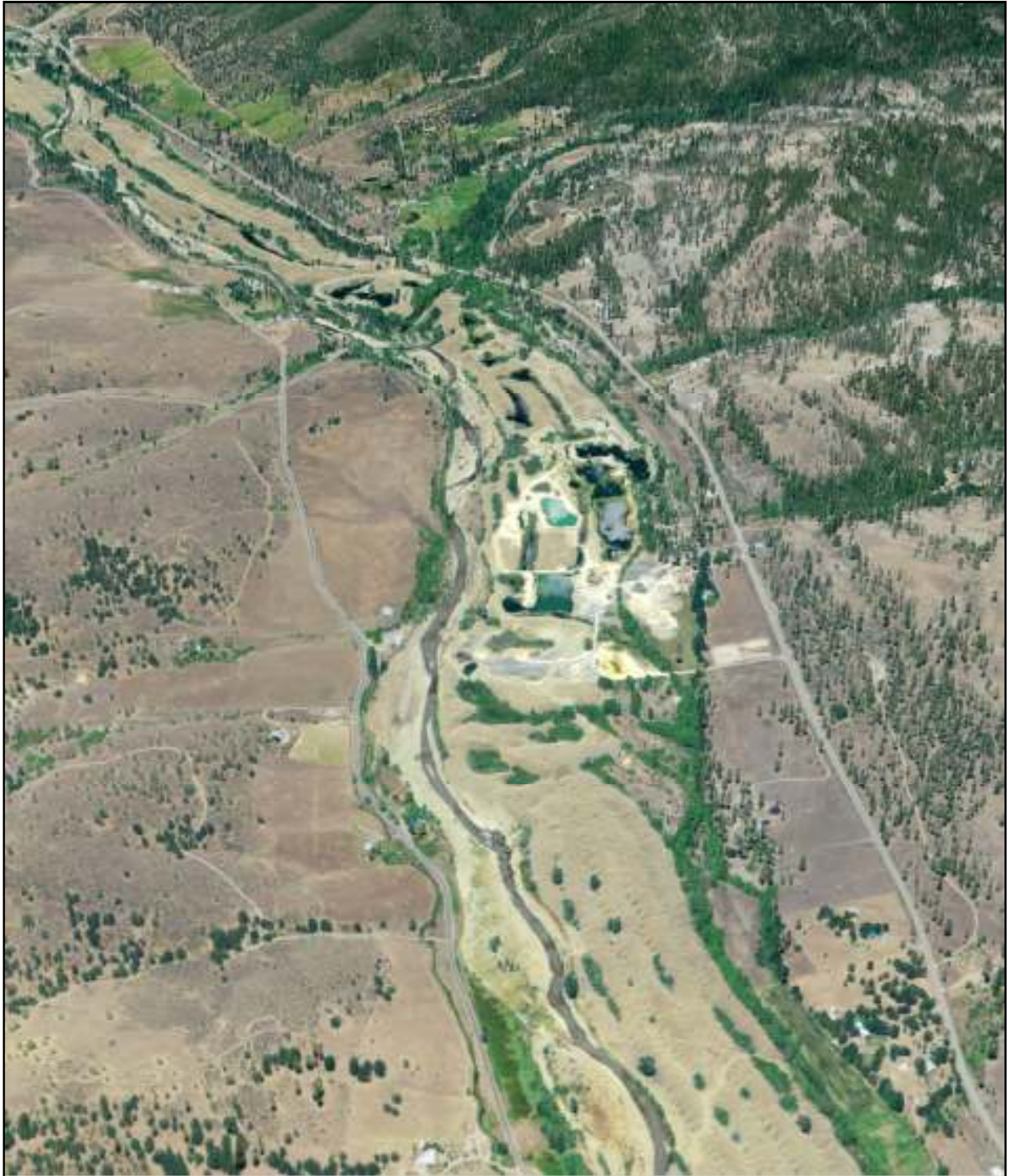
Figure 7.3. Scott River, downstream of Callahan, California. Image created by extracting RGB values from a NAIP orthophoto onto a three dimensional LiDAR point cloud.
