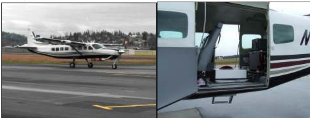
The Cessna Caravan is a powerful and stable platform, ideal for the mountainous terrain of the Pacific Northwest. The Leica ALS50 Phase II sensor head installed in the Caravan is shown on the right.
